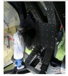
J-black coating in telescope cavity for long wavelength stray light control
