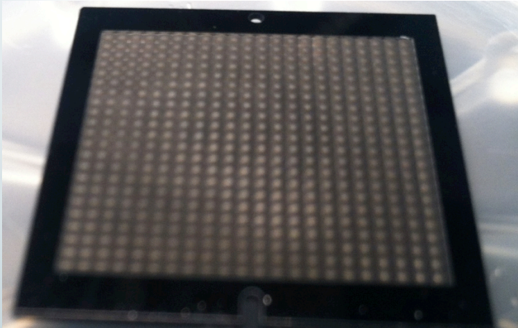
Laser etched square packed lens array
