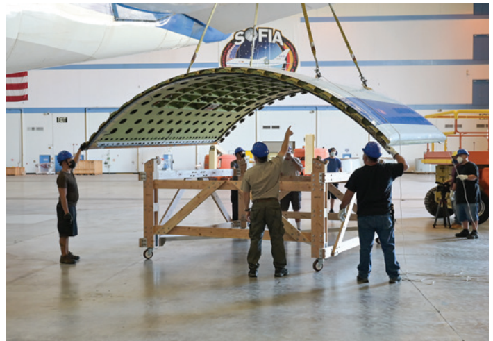
SOFIA undergoes annual maintenance during Fall 2021 at NASA's Armstrong Flight Research Center in California, including both routine aircraft maintenance and specialized procedures unique to the aircraft. One of the specialized procedures is maintenance of the upper rigid door that opens to allow the telescope to view the sky. In these images, the SOFIA team attaches the upper rigid door to a crane, then lifts and gently lowers the door onto a stand for inspection and servicing. (Top left, bottom right: Syd Meyers; top right, bottom left: NASA/Agnew)
