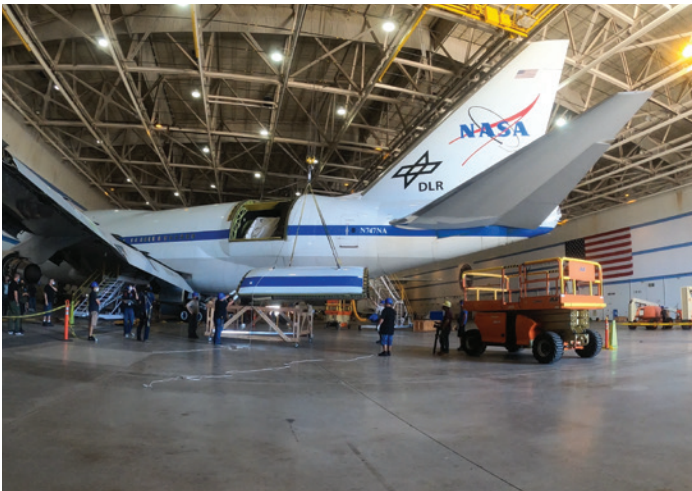
SOFIA undergoes annual maintenance during Fall 2021 at NASA's Armstrong Flight Research Center in California, including both routine aircraft maintenance and specialized procedures unique to the aircraft. One of the specialized procedures is maintenance of the upper rigid door that opens to allow the telescope to view the sky. In these images, the SOFIA team attaches the upper rigid door to a crane, then lifts and gently lowers the door onto a stand for inspection and servicing. (Top left, bottom right: Syd Meyers; top right, bottom left: NASA/Agnew)
