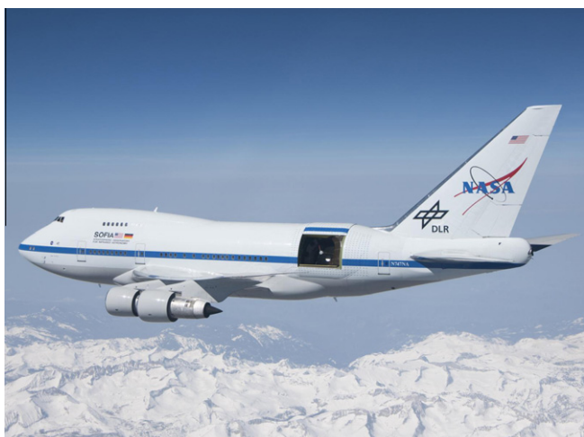
Fig. 1. With the sliding door over its 17-ton infrared telescope wide open, NASA's Stratospheric Observatory for Infrared Astronomy (SOFIA) soars over California's snow-covered Southern Sierras on a test flight on April 14, 2010.
