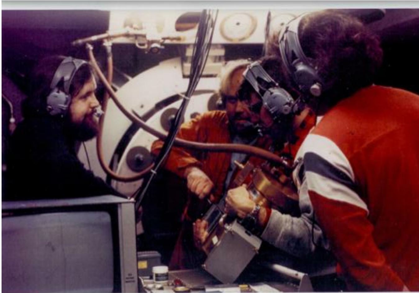
Figure C12. Graduate student Ian Gatley, Eric Becklin, Gerry Neugebauer, and Gordon Forrester (Caltech), 1976, making in-flight repairs to their far-infrared photometer.
