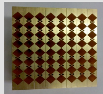
Stacked 1x8 Linear Arrays @ 350 GHz
