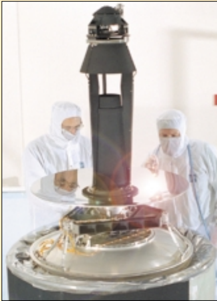
Technicians inspect SIRTf's infrared telescope, whose mirror is 0.8 meter in diameter. Courtesy of NASA/JPL/Caltech.
