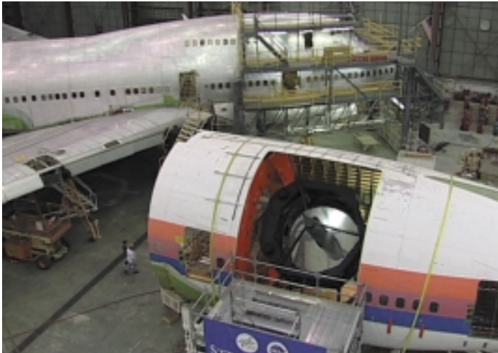
Left: The SOFIA 747 (rear) rests in a Waco, Texas hangar along with a cut-up section of a “donor” 747 housing a full-scale dummy telescope. Courtesy of L3 Communications. Right: Technicians test the cabin side of the telescope’s suspension assembly and Nasmyth tube. Courtesy of MAN-Technologies.
