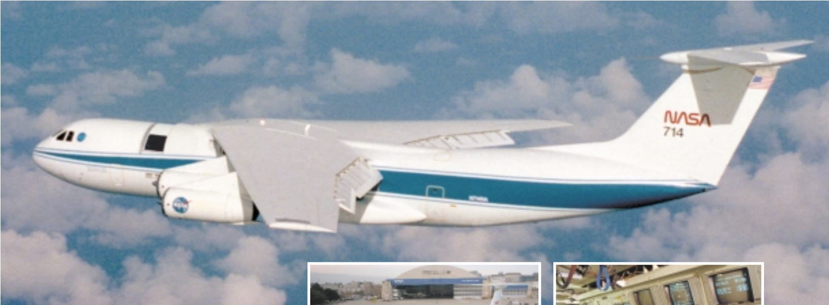
KAO represented a giant leap forward for airborne astronomy (note the telescope port in the top image). Right inset: KAO's Mission Director's console exemplifies the airplane's crowded interior.
