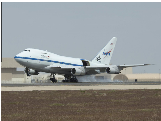
Fig. 13. The SOFIA 747 SP aircraft was put through an extensive series of test flights to evaluate performance over the entire operational envelope. Here, with the door to the cavity housing its 2.5-m infrared telescope wide open in a scheduled test to demonstrate that emergency door-open landings can be accomplished without dangerous control issues and/or contamination of the telescope cavity, Clipper Lindberg flares for landing at Air Force Plant 42 in Palmdale, Calif., after a test flight on April 14, 2010. (NASA Photo/Tony Landis).
