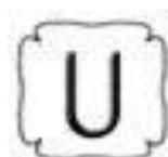
Figure 3.5-1: Example stamp for ASME Section VIII Division 1 pressure vessel (ref.: paragraph 3.5.3.5)
