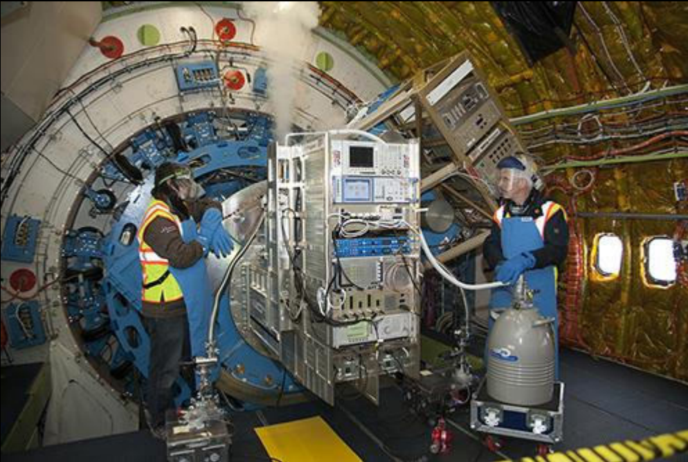
German REceiver for Astronomy at Terahertz Frequencies (GREAT)
