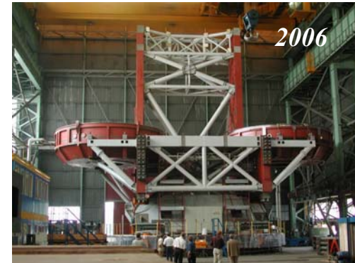
The LBT, Mt. Graham, AZ, 2 x 8.4-m on a 22.8-m single mount
