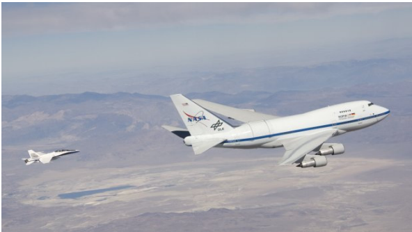
Figure 1-1. The SOFIA infrared observatory with chase plane during the first series of test flights to verify the performance of the modified Boeing 747SP. From the NASA Dryden Flight Research Center Photo Collection.
