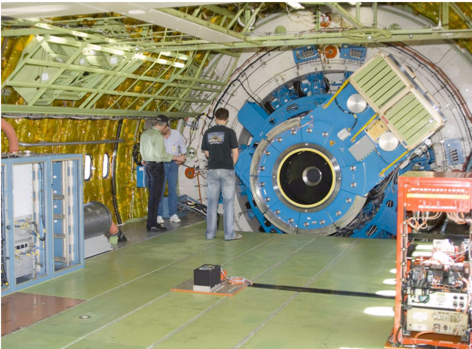
Figure 1-6. Main cabin looking aft toward the pressure bulkhead and telescope assembly.
