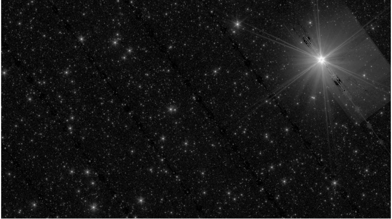
Figure 17: Example of pull-down latents in an IRAC [4.5] image centered at l=165.2^\circ , b=-0.45^\circ . Also note the frame pull-up near the bright source on the right.
