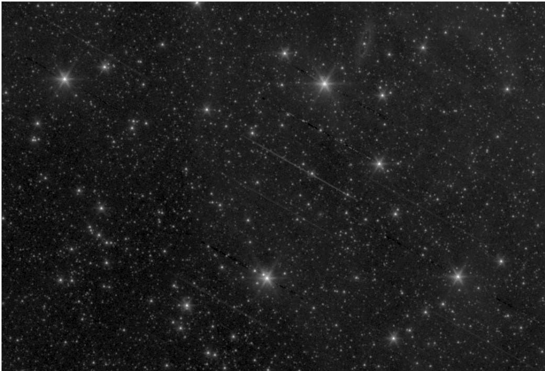
Figure 18: Example of column pull-ups in an IRAC [4.5] image centered at l=135.73^\circ , b=+0.92^\circ .
