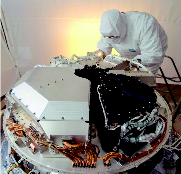
Fig. 3 Three Spitzer instruments installed on the base plate of the instrument chamber. The four modules of the IRS are seen in the background. In the foreground, the IRAC, with its black exterior, is to the right, and the MIPS to the left. The black area at the center of the base plate is the telescope focal plane into which the instrument pick-off mirrors protrude.
