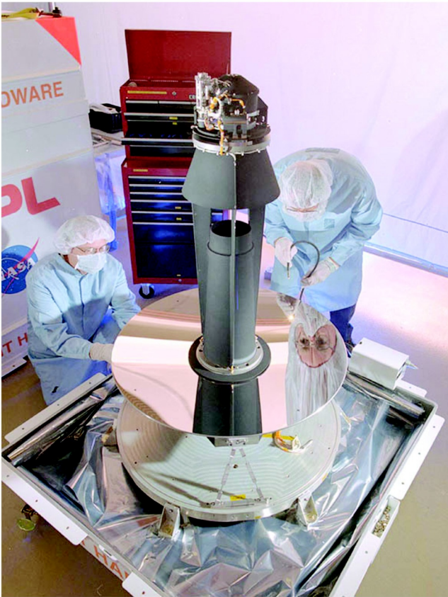
Fig. 1 Spitzer telescope. This picture shows the assembled optical system—primary mirror, metering tower, secondary mirror (not visible), and focus mechanism atop the tower.
