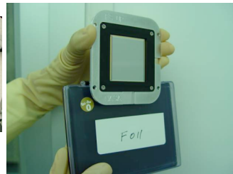
NIRSpec Microshutter Array Flight Candidate
