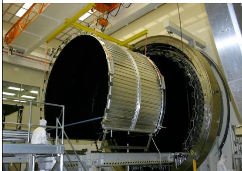
He Shroud Installation at MSFC X-Ray Calibration Facility (XRCF)
